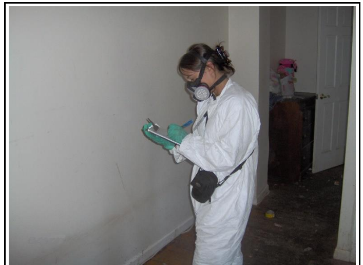
Collection of asbestos samples, City of Lebanon Bridge Street Project in Lebanon County; PennDOT Engineering District 8-0
